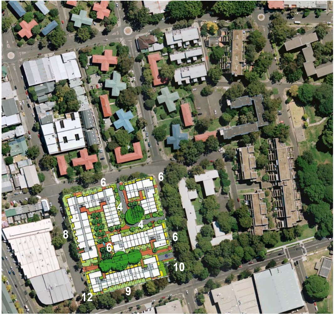
Figure 43. Sample Block 16 design by RWA superimposed on aerial photo (number of floors indicated)
