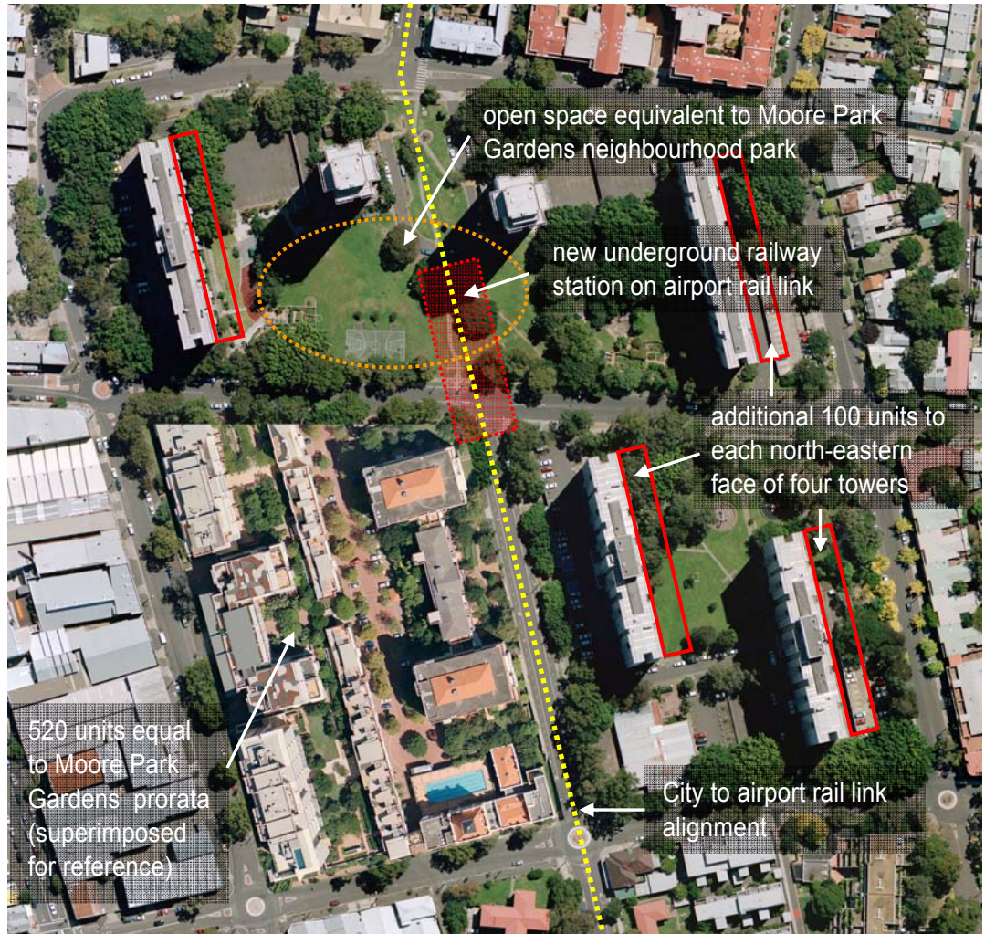
Figure 40. Concepts worth testing if railway station is located along George Street in Block 10.
