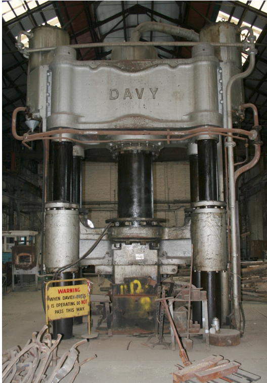
Figure 12 - Davy Press in Bay 1 North, Loco Workshops
