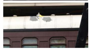
Photos taken on the 6th October 2007 show the damaged roof skin of carriage AAH19, parts of which were being blown away by the prevailing hot wind. Was this carriage fully checked out by RailCorp before they signed the release papers for the removal of these Heritage Listed Carriages from the protected Eveleigh Large Erecting Shop.
