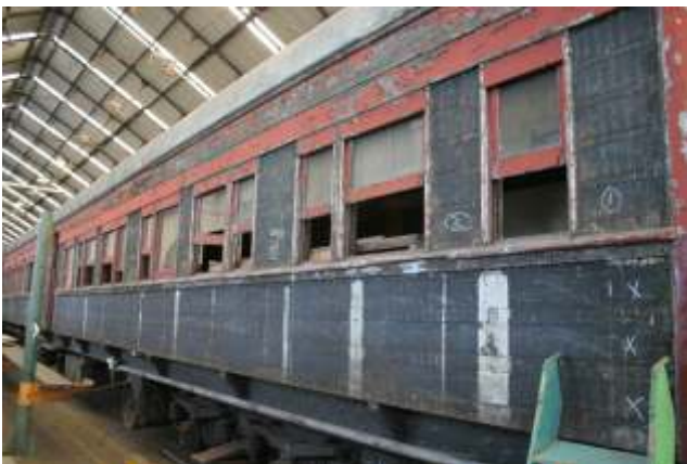
The non-repairable side panels have been removed
